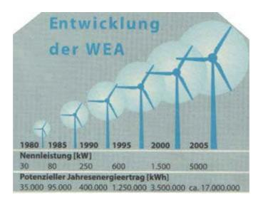
Here you can see the progress of efficiency of our windmills in the last 20 years. In 1980 we installed such little windmills which produced electricity for about 35 people. But today we install Five-Megawatt-Windmills which produce electricity for 17.000 people.
